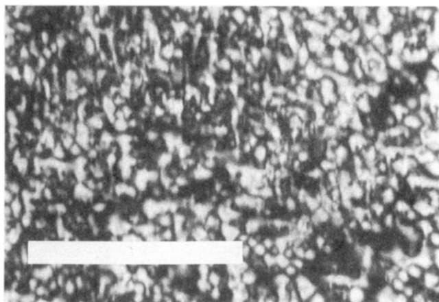
Figure 2. Threaded texture optical micrographs. Bar represents 100- \mu m marker.
